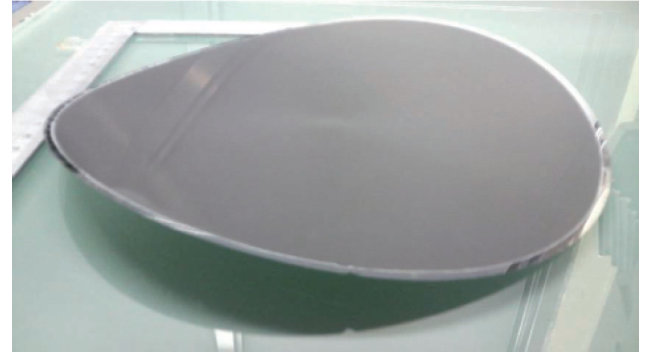
Figure 4: Blank moulded wafer warpage: Si - 100 \mu\text{m} , EMC - 200 \mu\text{m} (Takahashi et al., 2012).
